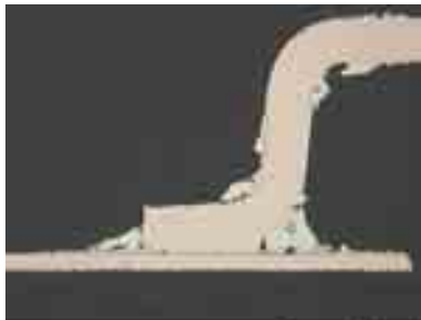
P-TQFP-100-1 on Au/Ni (SnAg3.8Cu0.7-after 4000 Cycles)
