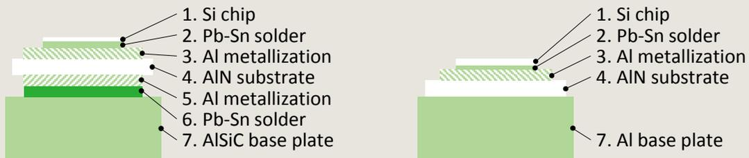
New base plate results in higher thermal conductivity between junction and case and an increased thermal-cycling performance
